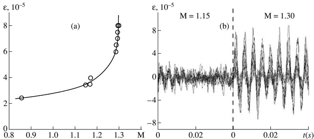
**Fig. 2.** (a) Amplitude of dynamic deformations of the plate as a function of the Mach number and (b) variation in dynamic deformations in time (the data from several strain gages are shown) in the mode  $M = 1.15$  (stability) and  $1.30$  (flutter).
