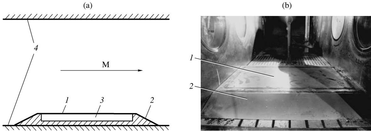
**Fig. 1.** (a) Experimental layout and (b) the model mounted in the tunnel. (1) Plate, (2) frame, (3) cavity, and (4) perforated tunnel walls.
