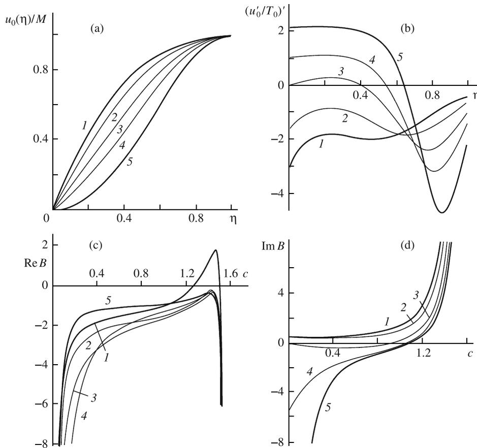
**Fig. 3.** Velocity profiles of decelerated and accelerated flows above a heat-insulated plate for parameters (4.2),  $M_\infty = 1.6$ , and  $Pr = 1$ : velocity profiles (a); generalized curvature (b);  $Re B$  (c), and  $Im B$  (d); curves (1–5) correspond to  $\beta = 2.0, 0.5, 0.0, -0.14$ , and  $-0.199$ , respectively.
