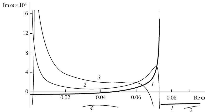
**Fig. 8.** Curve  $\Omega$  for profile 5 in Fig. 3. Vertical broken straight line corresponds to transonic transition,  $c = M_\infty - 1$ : curves (1–4) correspond to  $\delta = 0, 0.5, 1,$  and  $2,$  respectively.
