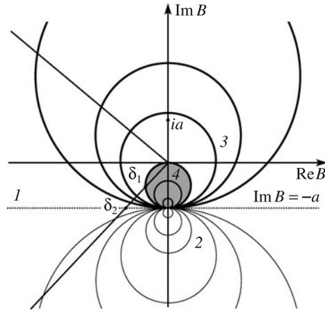
**Fig. 2.** Level lines of  $\text{Im}(A + B)^{-1}$ : straight line  $l$  corresponds to  $\text{Im}(A + B)^{-1} = 0$ ; curves 2 correspond to the family of lines below straight line  $l$  where  $\text{Im}(A + B)^{-1} > 0$ ; curves 3 to the family of lines above straight line  $l$  when  $\text{Im}(A + B)^{-1} < 0$ ; and 4 corresponds to the region in which  $\text{Im}(A + B)^{-1} < \text{Im}A^{-1} < 0$ .
