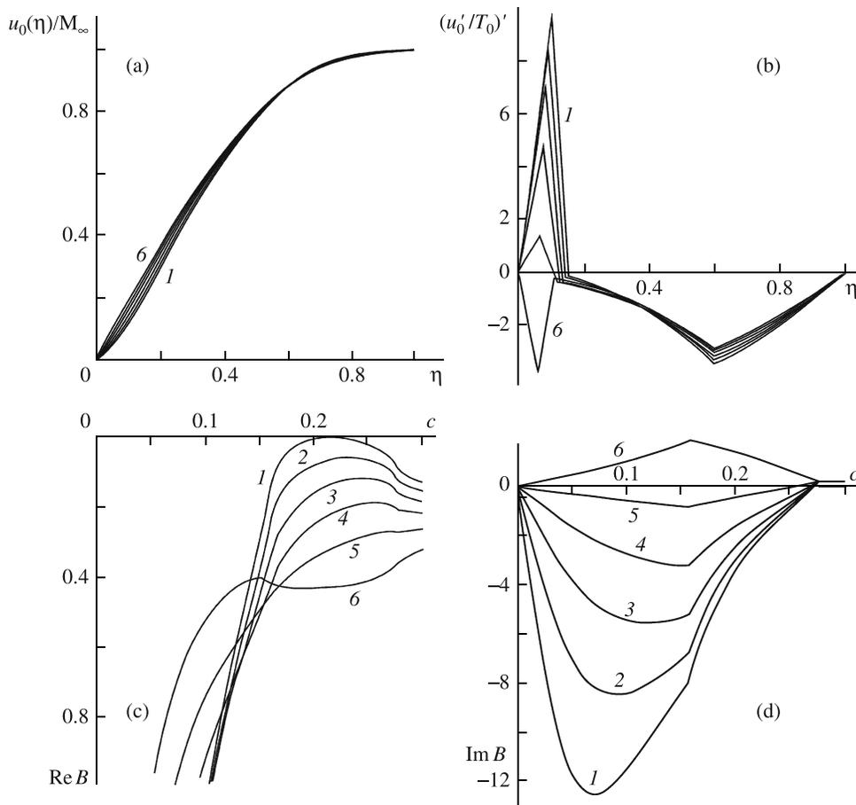
**Fig. 5.** Velocity profiles (5.2) for a heat-insulated plate and parameters (4.2),  $M_\infty = 1.3$ , and  $Pr = 1$ : velocity profiles (a); generalized curvature (b);  $Re B$  (c), and  $Im B$  (d); curves (1–6) correspond to  $s = 0, 0.2, 0.4, 0.6, 0.8$ , and  $1$ , respectively.
