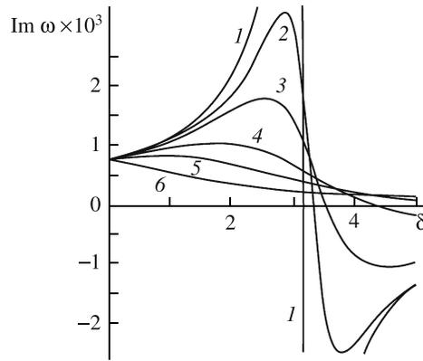
**Fig. 6.** Function  $\text{Im } \omega(\delta)$  for profiles (5.2) and parameters (4.2),  $M_\infty = 1.3$ , and  $k = 0.043$  ( $c \approx 0.21$ ): curves (1–6) correspond to  $s = 0, 0.1, 0.2, 0.4, 0.6$ , and  $1$ , respectively.
