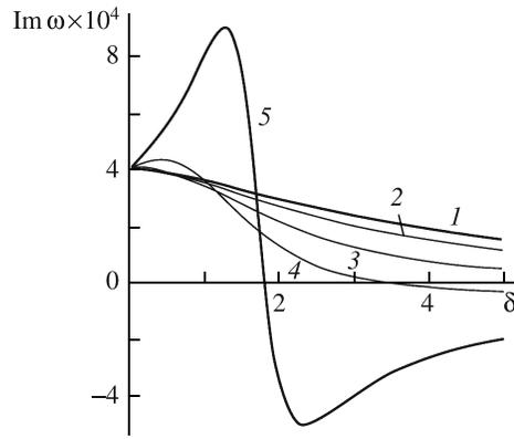
Fig. 4. Function  $\text{Im} \omega(\delta)$  for profiles (1–5) in Fig. 3 for parameters (4.2),  $M_\infty = 1.6$ , and  $k = 0.06$ .
