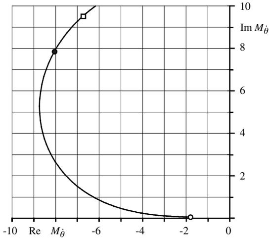
Fig. 6  $M_{\theta}(k_1)$  change when changing flow speed  $V$  from  $V = 10$  m/s (open circle) to  $V = V_{\text{div}} = 54.9$  m/s (filled circle) and further to  $V = V_{\text{div}} + 5 = 59.9$  m/s (square).
