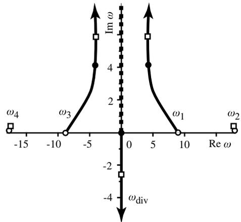
**Fig. 5** Eigenfrequency loci calculated through full unsteady aerodynamics when changing flow speed  $V$  from  $V = 10$  m/s (open circles) to  $V = V_{div} = 54.9$  m/s (filled circles) and further to  $V = V_{div} + 5 = 59.9$  m/s (open squares). Dashed curve shows the continuous spectrum.
