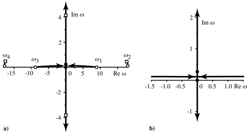
**Fig. 2** Eigenfrequency loci in quasi-steady approximation when changing flow speed  $V$  from  $V = 10$  m/s (open circles) to  $V = V_{div} = 54.9$  m/s (filled circles) and further to  $V = V_{div} + 5 = 59.9$  m/s (open squares): a) general view, and b) enlarged view around zero frequency.
