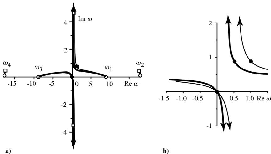
**Fig. 4** Eigenfrequency loci calculated with simplified unsteady aerodynamics with complex  $M_{\dot{\theta}}$  when changing flow speed  $V$  from  $V = 10$  m/s (open circles) to  $V = V_{div} = 54.9$  m/s (filled circles) and further to  $V = V_{div} + 5 = 59.9$  m/s (open squares); a) general view, and b) enlarged view around zero frequency.  $M_{\dot{\theta}} = -1.2 + i$  (bold lines), and  $M_{\dot{\theta}} = -1.2 + 2i$  (thin lines).
