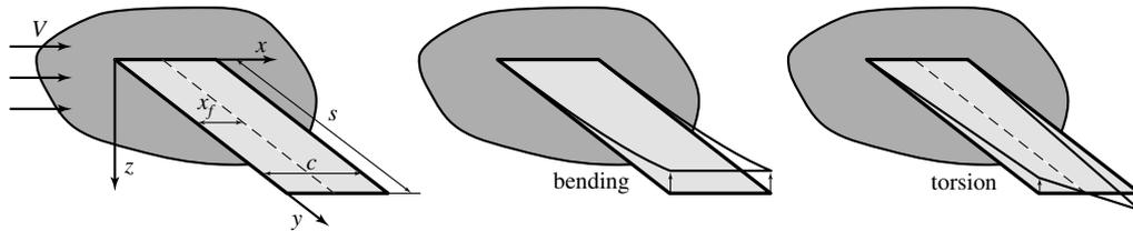
Fig. 1 Rectangular wing and its bending and torsional degrees of freedom.
