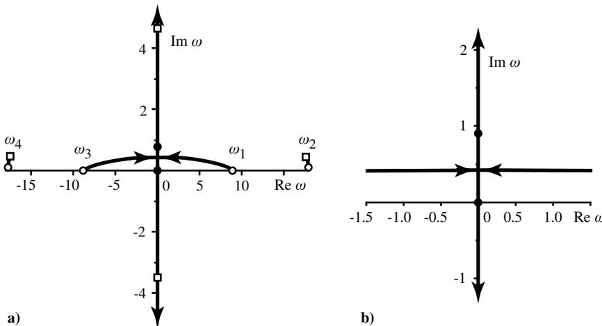
**Fig. 3** Eigenfrequency loci calculated with simplified unsteady aerodynamics with real  $M_{\dot{\theta}}$  when changing flow speed  $V$  from  $V = 10$  m/s (open circles) to  $V = V_{div} = 54.9$  m/s (filled circles) and further to  $V = V_{div} + 5 = 59.9$  m/s (open squares): a) general view, and b) enlarged view around zero frequency.
