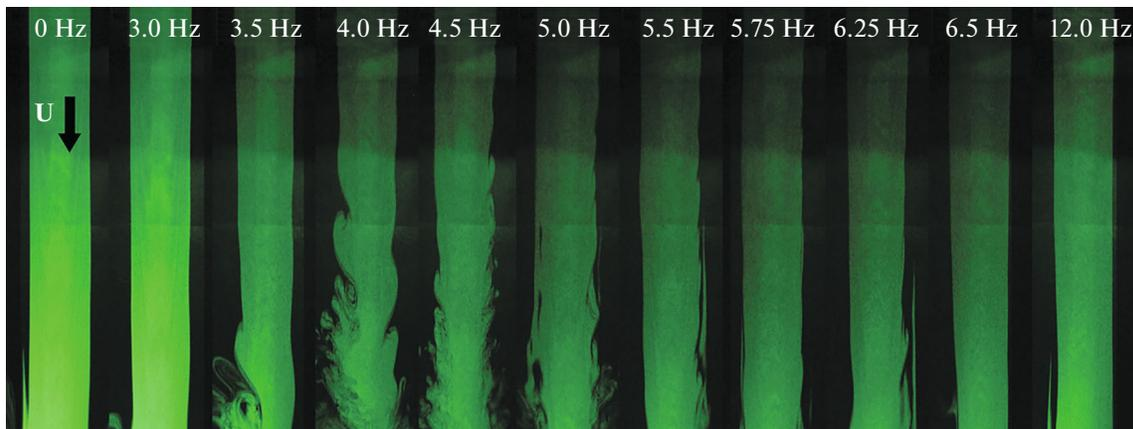
Fig. 3. Photographs of the jet in the section of the laser sheet at different vibration frequencies of ring no. 1.
