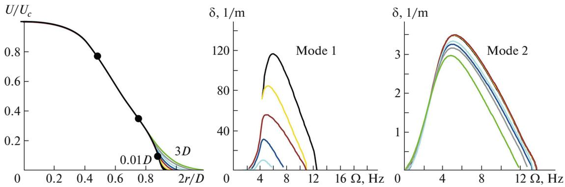
**Fig. 1.** Velocity profiles nondimensionalized to the maximal velocity and the jet radius at various distances from the jet beginning (the circles show the generalized inflection points of the initial profile); the growth rates versus frequencies for the modes of two branches of growing perturbations. The colors correspond to those of the velocity profiles and indicate different distances from the jet beginning.
