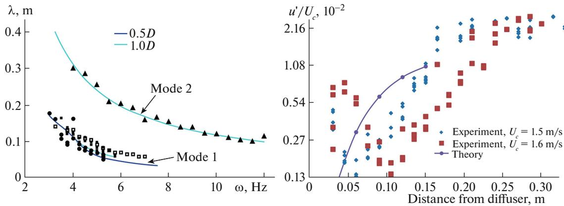
**Fig. 4.** Comparison between the experimental and theoretical dependences of the wavelengths  $\lambda$  on frequency. The symbols show the wavelengths obtained in experiments, and the curves represent the wavelengths obtained theoretically. Comparison of the theoretically established growth rate of perturbation with the frequency of 5 Hz and the highest amplitude of the relative velocity fluctuations  $u'/U_c$  on the distance from the beginning of the jet.
