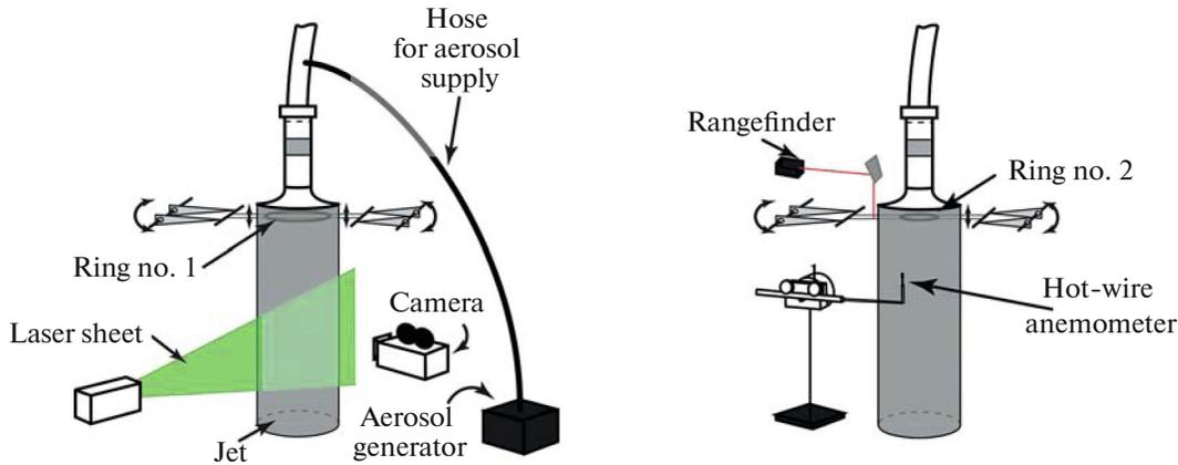
Fig. 2. Schematic representation of flow, the introduction of perturbations into the jet, the laser sheet, and the hot-wire anemometer with a rangefinder.
