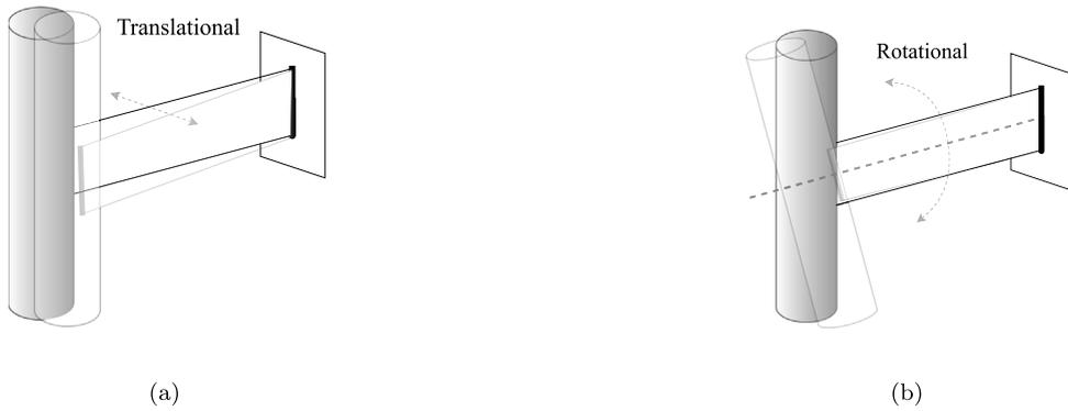
Fig. 1. Two predominant types of oscillation: (a) translational and (b) rotational of a circular cylinder attached to a rectangular beam.
