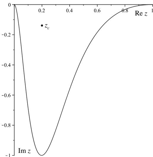
Figure 2: Integration path chosen for solving the Rayleigh equation for the velocity profile  $u_0(\eta) = M_\infty \sin(\pi\eta/2)$ ,  $M_\infty = 1.6$ ,  $c = 0.5 - 0.33i$ . The critical point is  $z_c \approx 0.20 - 0.14i$ .
