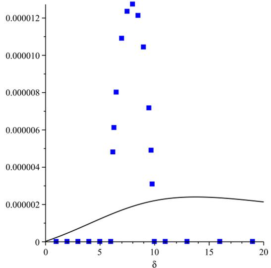
Figure 8:  $\text{Im } \omega(\delta)$  for  $k = 0.275$ . Numerical data are shown by points, analytical solution (10) is represented by the curve.
