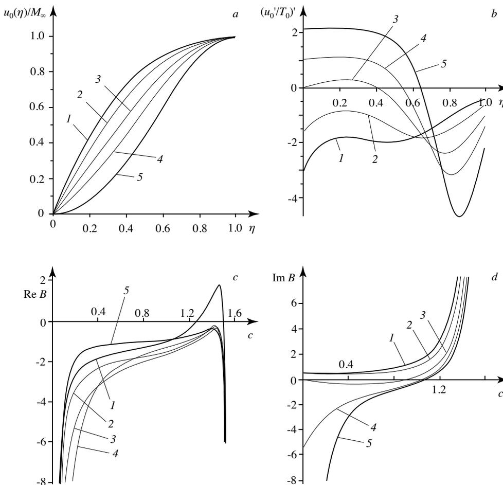
Figure 4: Velocity profiles for accelerating and decelerating flows over heat-insulated plate for parameters (13),  $M_\infty = 1.6$ ,  $Pr = 1$ : (a) velocity profiles, (b) generalised curvature, (c)  $Re B$ , (d)  $Im B$ . Curves 1–5 correspond to  $\beta = 2.0, 0.5, 0.0, -0.14, -0.199$ .
