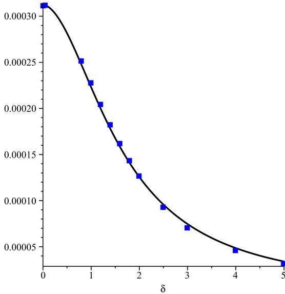
Figure 6:  $\text{Im } \omega(\delta)$  for  $k = 0.1$ . Numerical data are shown by points, analytical solution (10) is represented by the curve.
